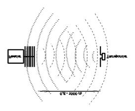
The energy arriving at the transponder is collected in the antenna aperture. The antenna aperture is a function of the operating frequency as shown in the table below
